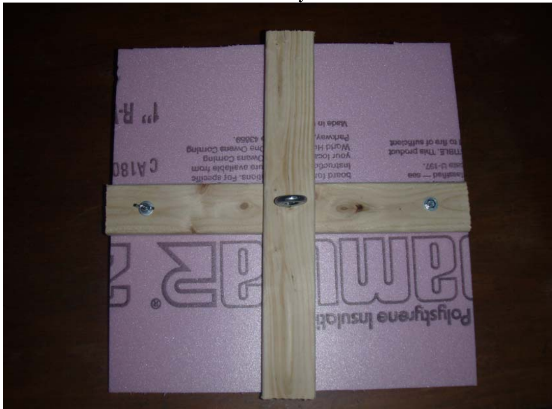
Figure 2. Underside of Sampler with Cross beams visible, eye bolt anchor hole visible and accessory bolts visible.
