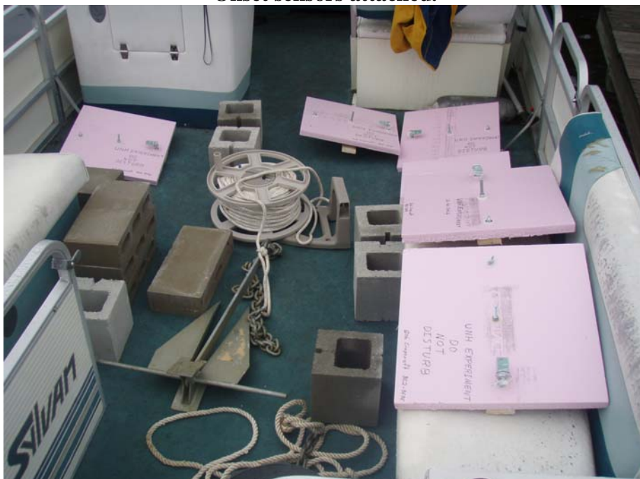
Figure 4. Periphyton Samplers awaiting deployment with Hobo Onset sensors attached.
